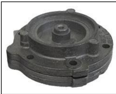
A. Top plate showing protrusion
